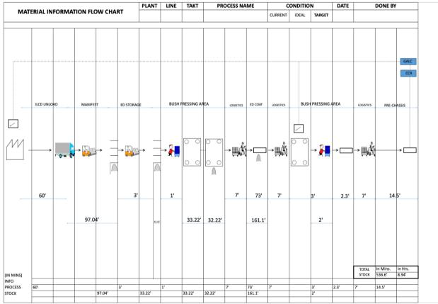
This is the current state of material flow from Supplier to Pre-Chassis, where it is supplied from the supplier and after entering the TKM it is manifested and sorted(stock), then it is stored at ED Storage(stock), then it is loaded in skid for ED(stock) at bush pressing area and sent to EDCoating(stock) after the coating it returns to bush pressing area and gets processed before being supplied to pre-chassis, where there are no stagnations in pre-chassis.
