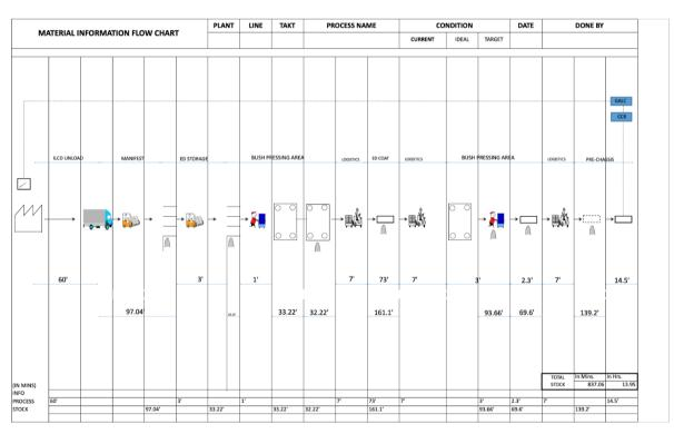
Current MIFC of the material flow from Supplier to Pre-Chassis:
