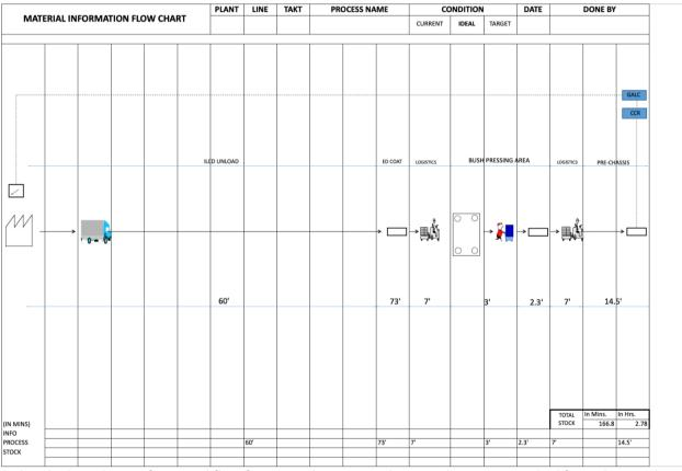
This is the ideal condition of material flow from Supplier to Pre-Chassis, where it is supplied from the supplier and after entering the TKM is manifested in the ED Coat area, then after thecoating it is sent to the bush pressing area and processed before being supplied to the pre- chassis.
